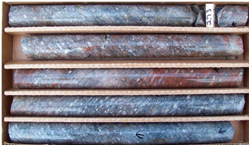
FIGURE 3.15 Drill core from the Leatherwood Granite showing highly sheared and mineralized granite. The average U_3O_8 percentage in this 10-foot core section is 0.679 percent. SOURCE: Wales (2010).
